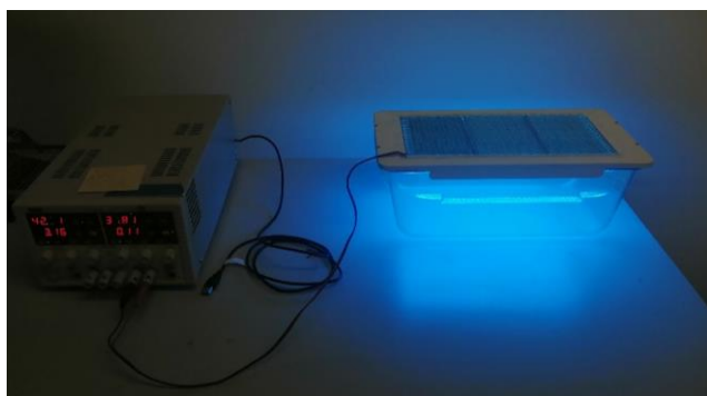
Figure 26: A cage lid designed for the non-invasive activation of photosensitive molecules in mouse models. This lid features an array of hundreds of LEDs positioned to uniformly illuminate the entire cage with a defined pattern of blue light.
